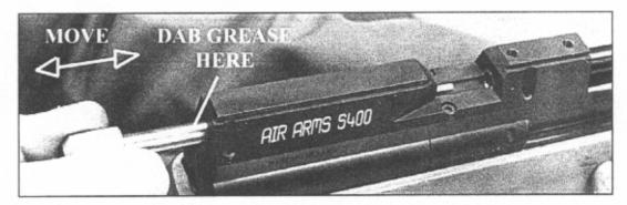
APPLY A SMALL DAB OF GREASE ON THE LOADING BOLT AND WORK-IN BY MOVING THE BOLT FORWARDS AND BACKWARDS. WIPE OFF EXCESSIVE GREASE. PREFERRED GREASE IS 'NAPIER G95 GUN GREASE'
